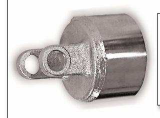
The COMPACT automatic clutch offers a level of implement overload protection not possible with other types of clutches. The compact, efficient design disconnects the power source from the drivetrain when overload occurs, and does not reconnect until the speed is reduced. During disengagement, the patented design minimizes damaging torque spikes and heat.
