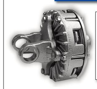
The MODULAR friction clutch is indispensable in certain agricultural implement applications. The friction clutch is the only torque limiter that has the ability to continuously transmit power (at a reduced level) while overloaded. This is valuable during start up of high inertia machines, as well as for leveling out torsional fluctuations due to high cyclic loads. The TorQmaster patented technology dissipates heat quickly, improving durability while protecting the machine.
