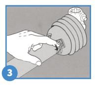
Turn the bushing until it engages into the guard.
