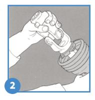
Slide guard half over drive shaft and insert bushing tabs into the openings in the guard.
