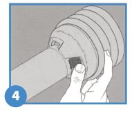
Push Easy Lock clip into position. The bushing and guard are now secure.
